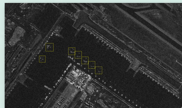
ICEYE Use of AI for SAR image for on-board object detection and classification
